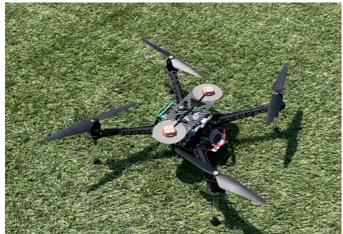
Fig. 4: Quadcopter equipped with a RadioLion
