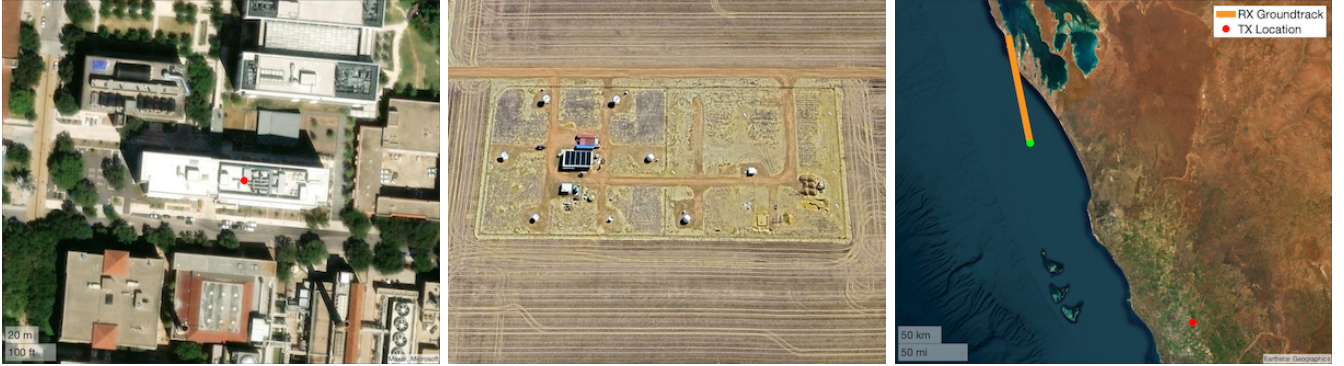
Fig. 3: The UT RNL provided a baseband binary file containing an ensemble of GNSS spoofing signals that would spoof a target receiver to the top of the former Aerospace Engineering building in Austin, Texas (left). This spoofing file was transmitted on a slice of S-band owned by Spire Global from a ground station located in Perth, Australia (middle). An overhead LEO satellite performed a 20 second raw capture (right).
