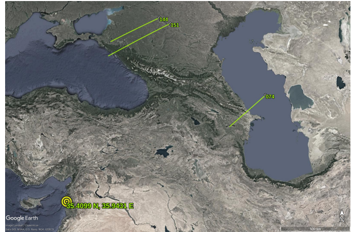
FIGURE 3 Ground tracks for interference-affected captures on days 74, 144, and 151 of 2018. Each capture spans approximately 70 seconds. The estimated transmitter location is marked on the west coast of Syria.
